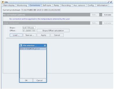
The proper correction factor depends on air-flow rate and 535 l/hr is the calibrated rate. For low temperature using the LN2 evaporator, the flow is determined by the heater percentage and 40% is the calibrated rate.
