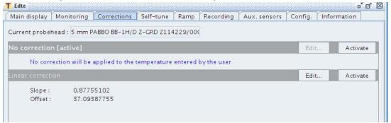
Then, click "load..." and select the file 300-373K@533.jd.cor or 200-293K@40%.jd.cor, as appropriate. Click apply and then click Activate on the linear correction line. The blue message "No correction with be applied..." under the grey No Correction remains but that is not important. Look ONLY at the grey lines for which mode is active. To disable, click Activate on the No Correction line.
